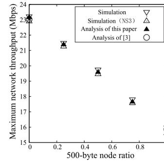
**Fig. 3** Maximum network throughput as a function of ratio of 500-byte node number.
