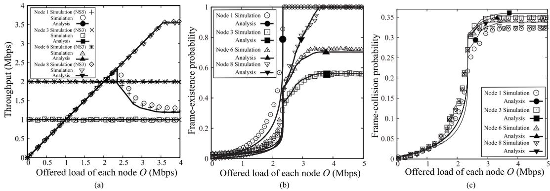
**Fig. 6** Network characteristics as a function of offered load of each node for Scenario 4. (a) Throughput. (b) Frame-existence probability. (c) Frame-collision probability.
