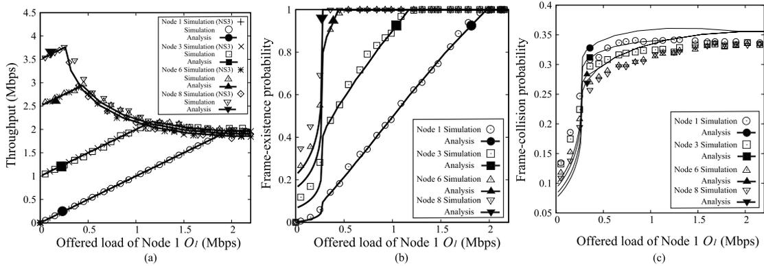
**Fig. 5** Network characteristics as a function of offered load of Node 1 for Scenario 3. (a) Throughput. (b) Frame-existence probability. (c) Frame-collision probability.
