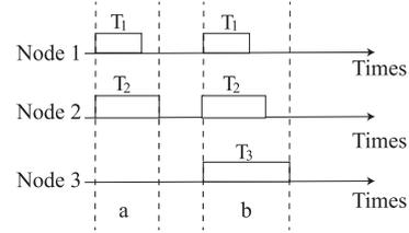
**Fig. 2** Example of frame-collisions due to concurrent-frame-transmission.
