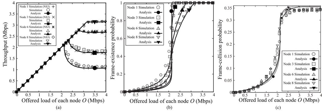
**Fig. 4** Network characteristics as a function of offered load of each node for Scenario 2. (a) Throughput. (b) Frame-existence probability. (c) Frame-collision probability.
